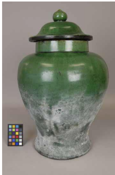
Deposit on covered jar from exposure to polyester polyurethane foam during exhibit. ©The Metropolitan Museum of Art. Image retrieved from AIC News v. 37 n. 1 (2012)
